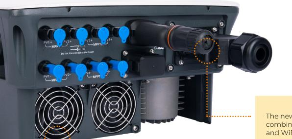
Inverters reduce output power at high temperatures in order to prevent hardware damage. That's why a **high-quality coolingsystem is essential for bigger inverters.** The fans of the 3-phase ensure optimal temperature management inside the inverter by adjusting their speed to any ambient temperature changes.
